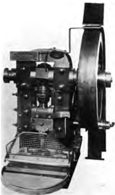
Fig. 4. Press tripped by Safety Gate.
